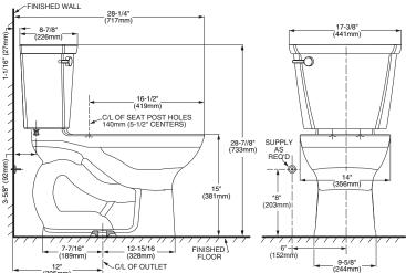
NOTES: THIS TOILET IS DESIGNED TO ROUGH-IN AT A MINIMUM DIMENSION OF 305MM (12") FROM FINISHED WALL TO C/L OF OUTLET.
