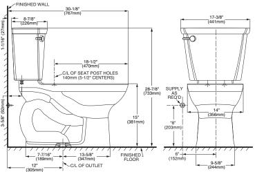
NOTES: THIS TOILET IS DESIGNED TO ROUGH-IN AT A MINIMUM DIMENSION OF 305MM (12") FROM FINISHED WALL TO C/L OF OUTLET. SUPPLY NOT INCLUDED WITH FIXTURE AND MUST BE ORDERED SEPARATELY. \* DIMENSION SHOWN FOR LOCATION OF SUPPLY IS SUGGESTED.
